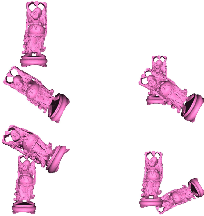
Figure 6.15: Our sphere-method uses a fixed rotation for every cycle. The moving object is rotated around the fixed object. After a cycle is finished, the rotation is changed.
