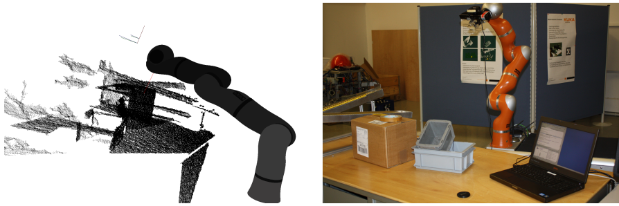
Figure 7.10: A typical point cloud recorded by the Kinect and the polygonal model of the LWR. The red line denotes the minimum distance between the LWR and the point cloud (left). The complete setup of our application: The KUKA Omnirobot with a head mounted Kinect in front of a workspace (right).
