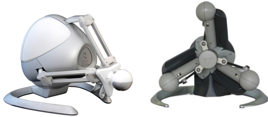
Figure 7.19: The haptic devices that we used in our evaluation: the 3 DOF Novint Falcon (left) and the 6 DOF Haption Virtuose 6D Desktop (right).
